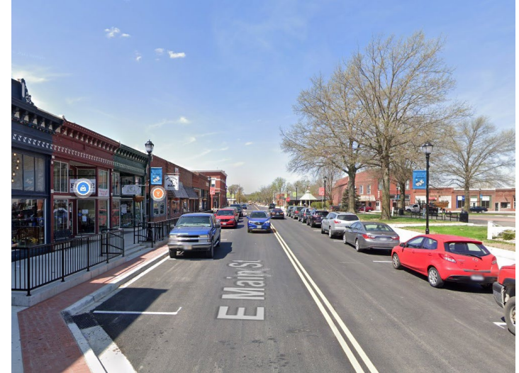
Narrow lane widths on Main St. help provide space for a safe and comfortable walking environment
